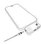
The headphone monitoring port has a driver and can directly drive headphones with an impedance of less than 36 ohms for real-time monitoring.
