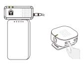
3 Connect the transmitter and receiver of the EM4.
